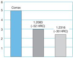
Uddeholm Corrax will withstand attacks from most corrosive plastics and diluted acids.
