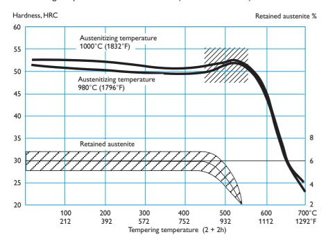
Above tempering curves are obtained after heat treatment of samples with a size of  $15 \times 15 \times 40$  mm, cooling in forced air. Lower hardness can be expected after heat treatment of tools and dies due to factors like actual tool size and heat treatment parameters.
