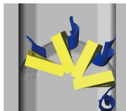
Proper chip control eliminates recuts and premature insert failure
